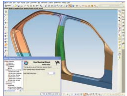
NX Body Design includes tools for creating a vehicle body side door opening.
