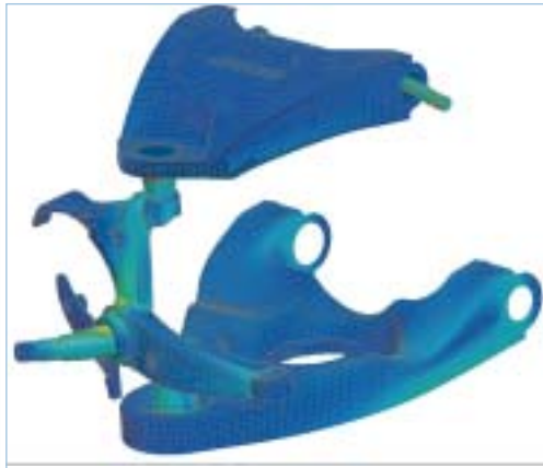
Figure 3. Analysis tasks that choke other systems can be performed with relative ease in Unigraphics NX 2. Stress analysis of this automotive suspension uses both shell and solid elements.
