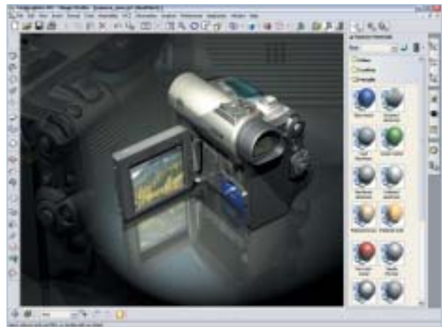
Figure 4. Once you set up a scene, materials, and lights, an optional module performs photorealistic rendering of concepts or finished models.
